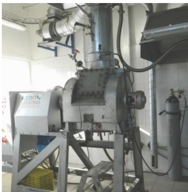
Fig. 2. Mixed dryer of semi-pilot testing unit.
