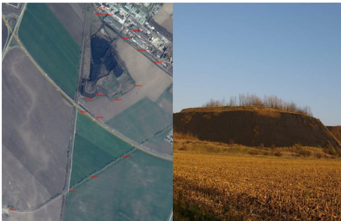
Fig. 1. Ground water monitoring net (red labels) in the surrounding of leach residue pile; southeastern view at the denuded part of leach residue pile (on the right)
