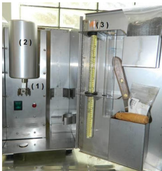
Fig. 1. Testing retort – (1) retort chamber, (2) condenser, (3) cylinder for condensate.
