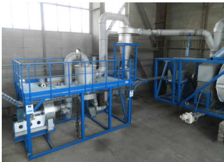
Fig. 5. Off-gas pretreatment module of continuous thermal desorption pilot unit.
