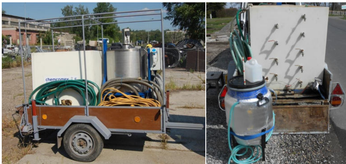
Fig. 1. Mobile system of IRON Technology (left) and its anaerobic reactor (right)
